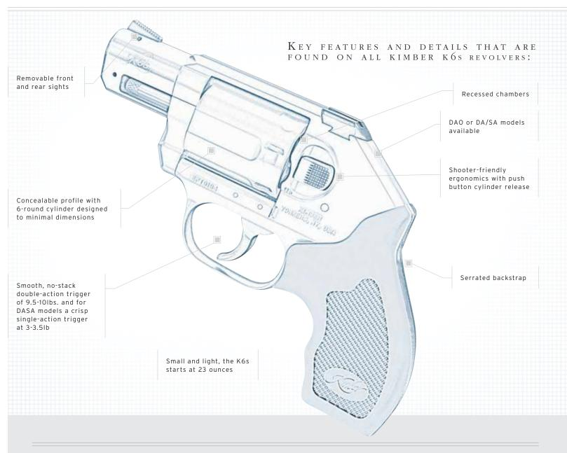
THE KIMBER K6s<sup>™</sup> IS AMONG THE MOST ACCURATE, shootable and dependable compact revolvers available today. Delivering on size and power, the K6s is the smallest 6-shot revolver on the market today that is specifically designed to fire .357 Magnum defensive
